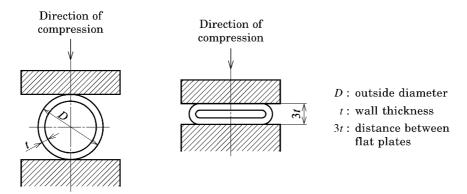
Figure 2 Flattening test
